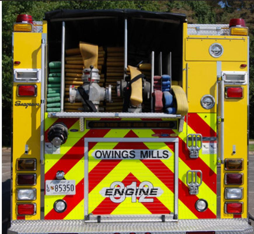
packed starting at the rear of the hose bed on either side. With the hose on its side, start laying the hose from the back corner of the hose bed along the hose bed walls until you reach the other corner. Once you reach the other corner, fold the hose back on itself and follow the hose back to the starting corner, forming a horseshoe.
